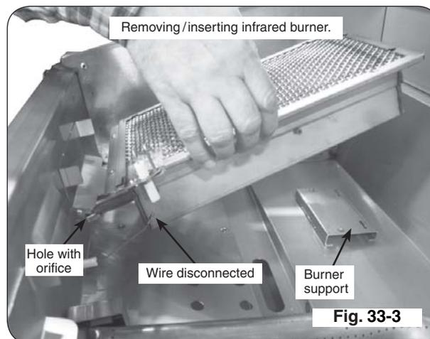
4. Using a  $\frac{1}{2}$ " deep socket, remove the orifice from the valve. Access this through the hole in the forward firebox plate (see PARTS LIST and Fig. 33-3).
