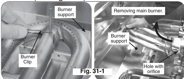
3. Using a 1/2" deep socket nut driver, remove the orifice from the valve. Access this through the hole in the forward firebox plate inside the grill (see PARTS LIST and Fig. 31-1).
