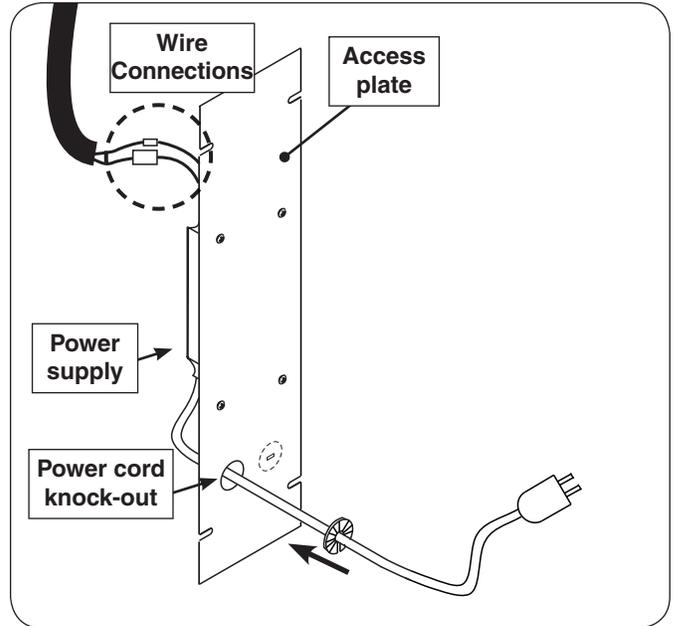
**Fig. 14-1** Access plate view & orientation
