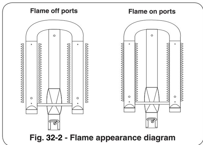
the air shutter until the flames appear to burn while touching the burner ports (Fig. 32-2). If flames are a lazy yellow, open the air shutters until the flame is mostly blue.
