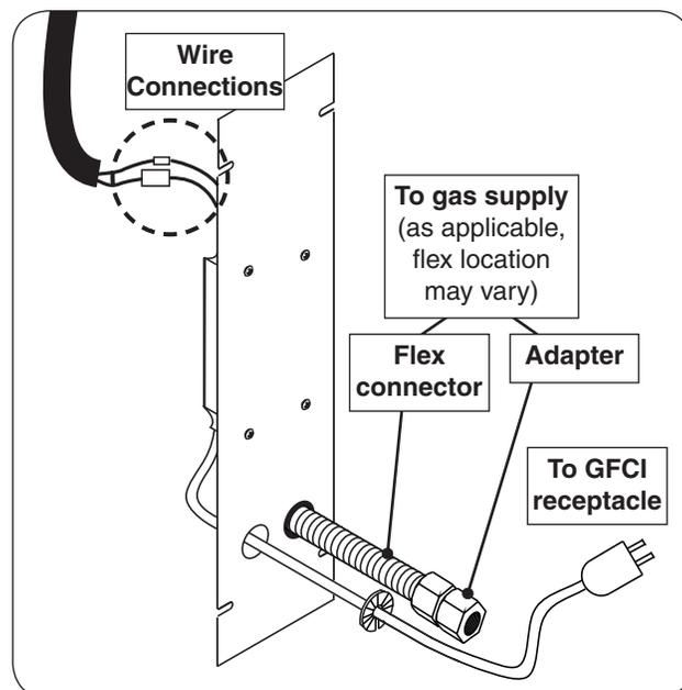
Fig. 13-1 Connect: Gas, Wires, Plate, Power
