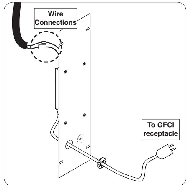
**Fig. 16-2** Connect: Wires, Plate, Power
