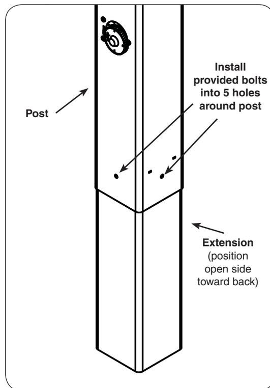
**Fig. 15-1** Install extension to post
